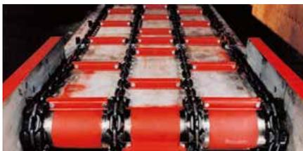
Armoured Chain Conveyor type PKF
