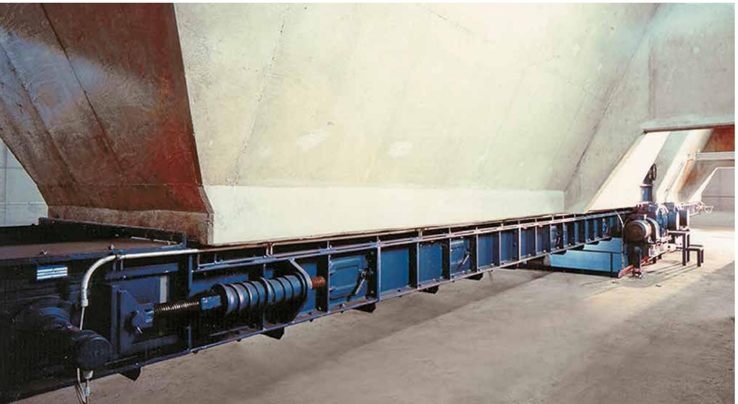
Hopper discharge with Armoured Chain Conveyor
