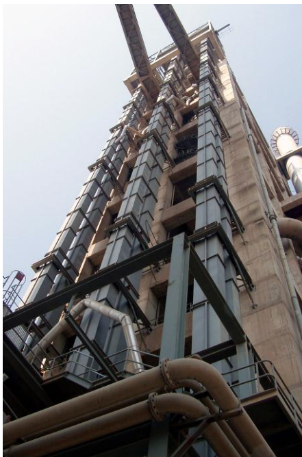
Example of an AUMUND Belt Bucket Elevator (© AUMUND)
